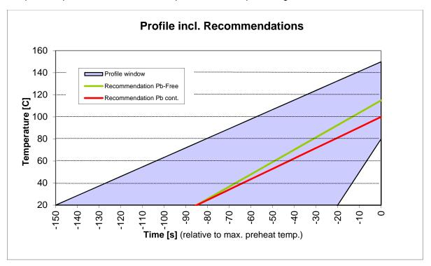
**DO NOT:** Use too high pre-heat temperatures as this will degrade the flux performance.
